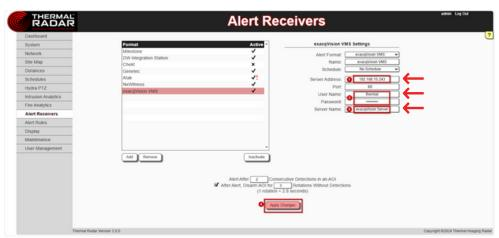
Navigate to Alert Receiver and select the Exacqvision VMS alert from the list
